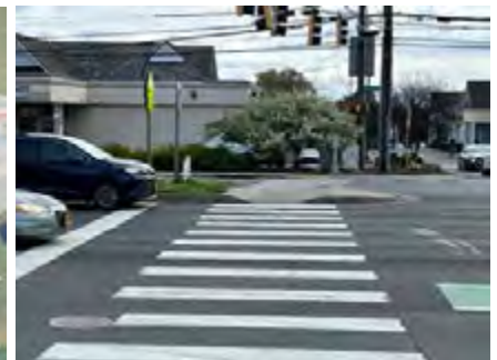
Crossing a six lane corridor with signage, high visibility crosswalks, and deeper median nose, Bethesda, MD
